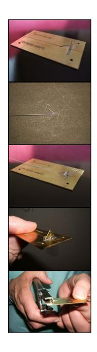
The 180 jig assembled. Use solder holes underneath to join the 2 levels together.
